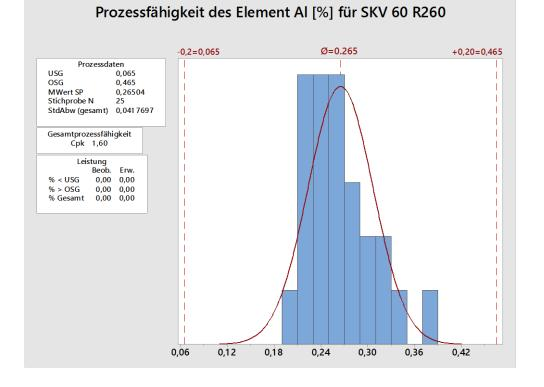
Due to a capable behavior of all elements with regard to the EN 14730 the **4**<sup>th</sup> **step Improvement** was not necessary...
